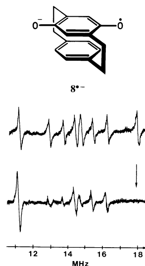
Figure 1. ^1\text{H} -ENDOR spectrum of the radical anion 8^{\bullet-} in DME/kryptofix® 222 at 220 K together with a general triple resonance spectrum, pump frequency 17.87 MHz
